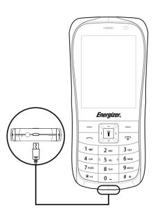
Connect battery charger to your phone and plug into the socket.
