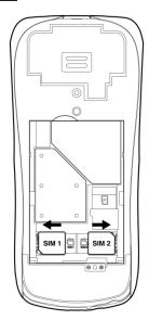
Place the SIM card with the chip facing downwards and slide it into its housing. Make sure that it is correctly inserted. To remove the card, press it and slide it out
