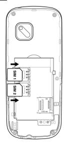
Place the SIM card with the chip facing downwards and slide it into its housing. Make sure that it is correctly inserted. To remove the card, press it and slide it out
