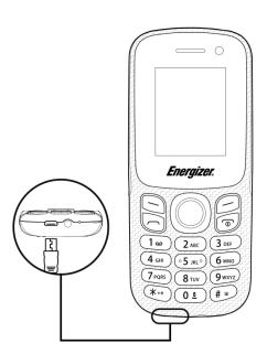
Connect battery charger to your phone and plug into the socket.
