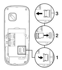
Place the microSD card with the chip facing downwards and slide it into its housing. Make sure that it is correctly inserted. To remove the card, press and slide it out.
